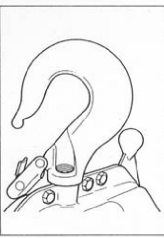
Fig. 11 - Machine anchor hook with catch in open position
