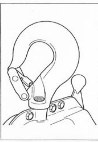
Fig. 12 - Machine anchor hook with catch in closed position.
